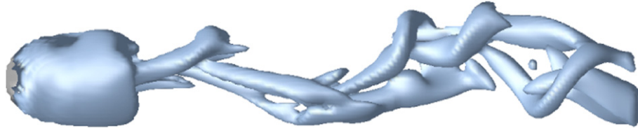
Fig. 5. yz view of the vortical structures behind single sphere at Re = 600 , steady inflow with flow direction from left to right.
